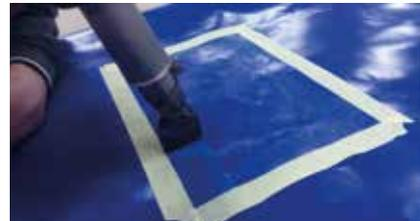
*Heat the surfaces treated with glue using a dryer (industrial or household) until the glue starts to bubble*
