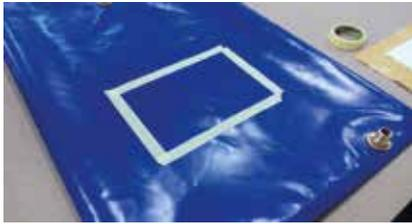
*Designate the perimeter for patch using the adhesive tape and degrease the surface. If necessary, abrade the perimeter of damage with a sandpaper.*
